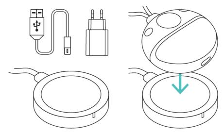
• If the charger's indicator diode doesn't go to green and the sensor's LED does not flash, adjust the sensor position on the charger.
