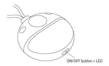
To start the sensor, **press for 1 second** the button located on its top. The sensor vibrates and the LED will flash rapidly in blue (1 flash per second for 90 seconds) signaling the possibility of pairing a phone.
