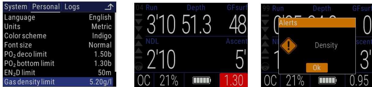
Examples of alarms with programmable thresholds in the "Personal" menu
