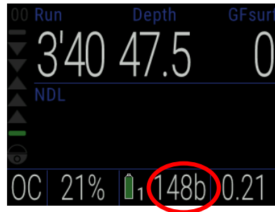
Illustration of the gas pressure available in tank N° 1 (pressure sensor n° 1): 148 bar
